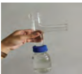
Cleaning sampling probe
