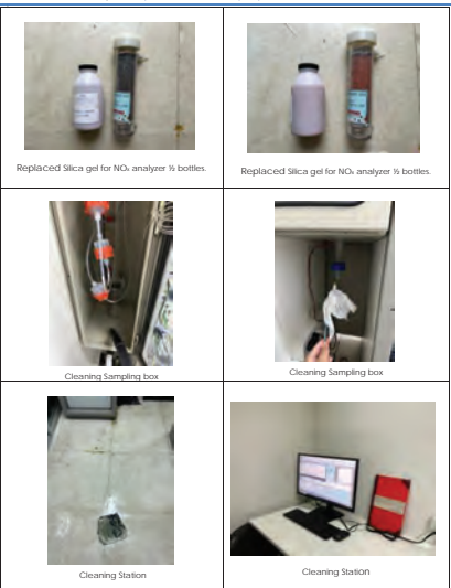
Replaced Silica gel for NOx analyzer ½ bottles.
