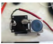
Clean diaphragm pump NOx analyzer
